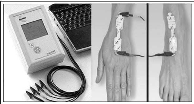
Figure 1. ImpediMed SFB7 Device and electrode placement on dry skin of dorsum of hand and foot. Courtesy of ImpediMed, Inc.
